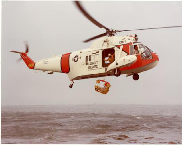
Stratford, CT – The Sikorsky HH-52A Seaguard, the first helicopter with a flying-boat hull. US Coast Guard photo.
