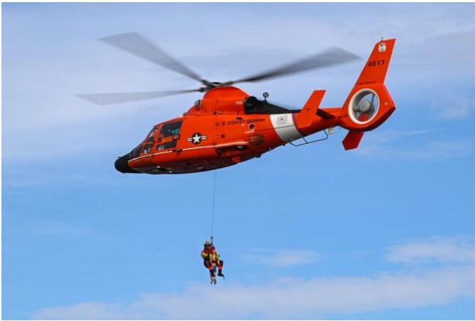
Aviation Training Center Mobile – An MH-65 Dolphin, recognizable by its enclosed fenestron tail rotor. US Coast Guard photo.
